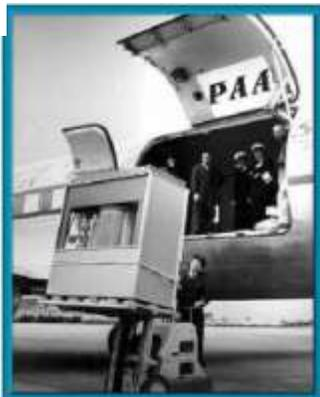
Geoff took us through the history of the hard disc drive, showing the first one: **In September 1956 IBM launched the 305 RAMAC, the first computer with a hard disk drive (HDD). The HDD weighed over a ton and stored 5MB of data (see picture left).**
